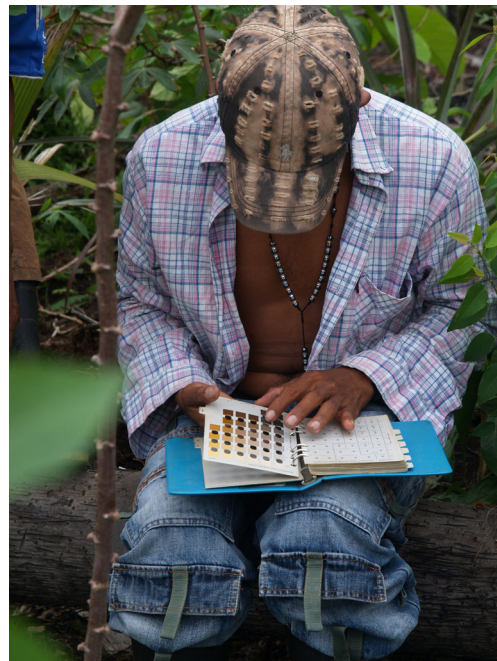
Fig. 2 Indigenous participant assessing the color of a collected soil sample using the Munsell soil color chart. Photo: Gerard Verschoor
